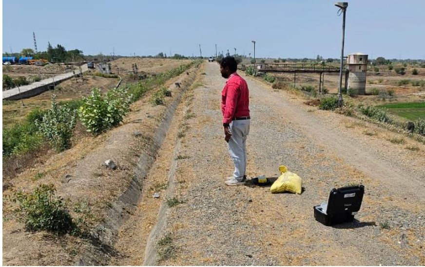
Vibration Monitoring on Top of Left Side Embankment during Actual Blasting
