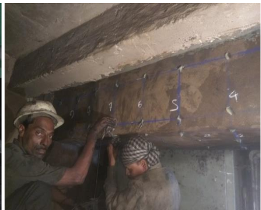
Beam Structure where opposite faces are not accessible (Indirect)
