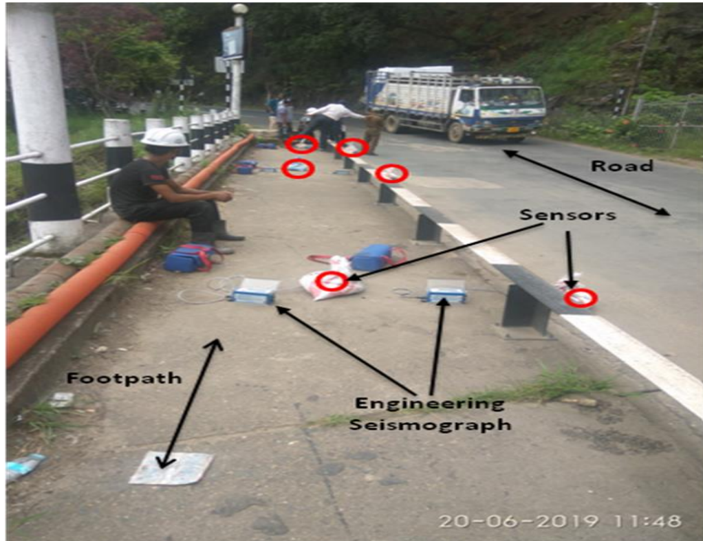
Schematic Diagram Showing Vibration Monitoring Points at Different Locations on Top of Umiam Dam, Meghalaya
